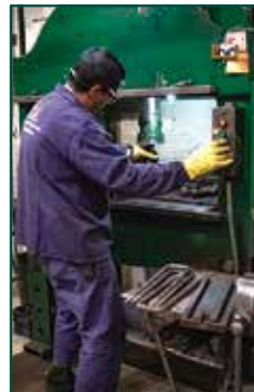
3. Hydraulic press for U-bolt clamps straightening
