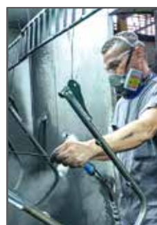
5. Production floor, electrostatic paint booth
