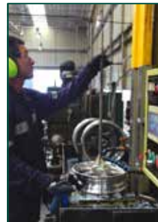
4. Motorcycle wheels line, manufacturing of internal groove
