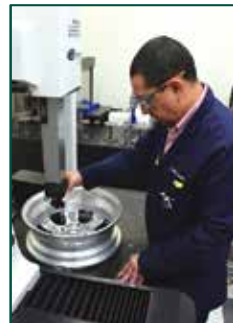
3. Quality process, measurement with CMM
