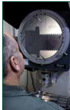
4. Laboratory area - profile projector
