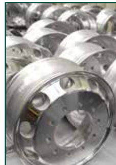
5. Finished product, 22.5" wheel for tractor unit
