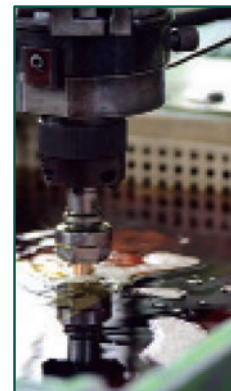
5. Erosion process of steel plates
