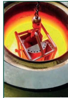
5. Heat treatment for cementing (Gcv2 furnace)
