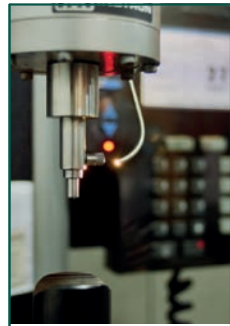
3. Durometer (Quality Inspection Laboratory)
