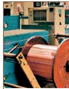
4. Centelsa wire bunching process
